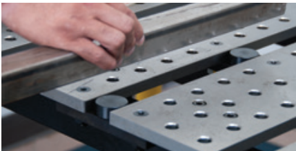
Mount the Channel Block and insert the Rest Button to create a continuous work surface over the table slot.
