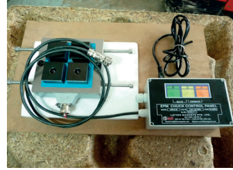
Double-Mag Fixture for Flange Clamping
