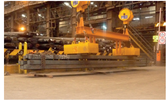
25 Ton Billet Lifter undergo load test
