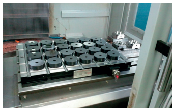
Metal-top Turbo Max-Mill 600 x 400 with round extension blocks
