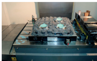
Standard 75mm Turbo Max-Mill 600 x 600 completed machining
