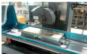
Electromicro Electromagnet on Grinding machine
