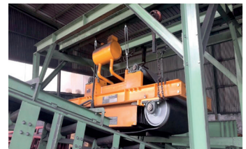
Oil-cooled Self-Cleaning EM Separator
