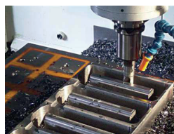
Machined out of solid body
