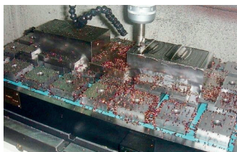
Standard 75mm Turbo Max-Mill 800 x 400 in machining operation
