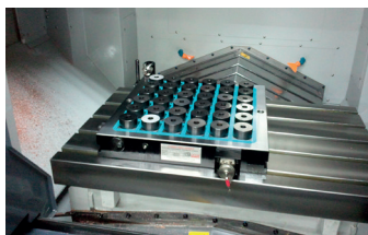
Standard 50mm Turbo Max-Mill 400 x 400 with round blocks
