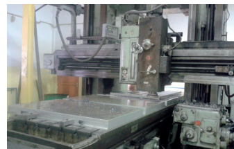
Conventional milling with four Turbo Max-Entry magnetic tables
