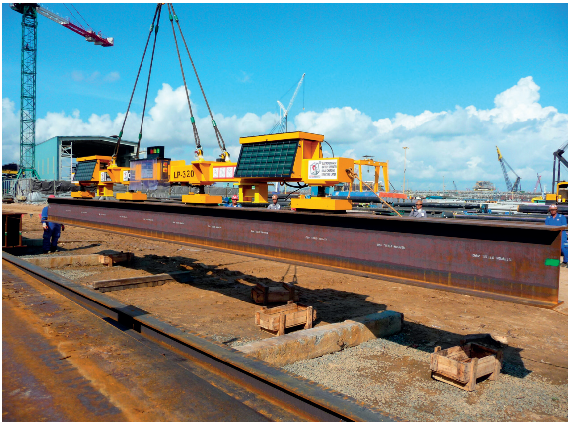
Solar Cell charging Battery Powered 5 Ton profile lifting system
