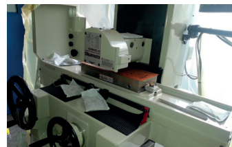
NeoEDM Grind Permanent Magnet table on Grinding machine
