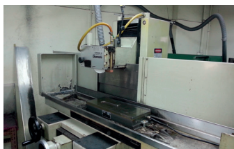
Electrogrip Electromagnet table on a Grinding machine
