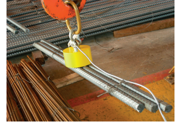
EM Circular Pot for profile lifting
