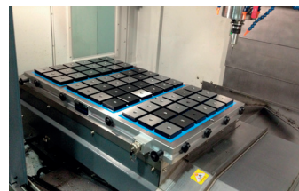
Turbo Max-Mill Standard model 1000 x 600 in a VMC
