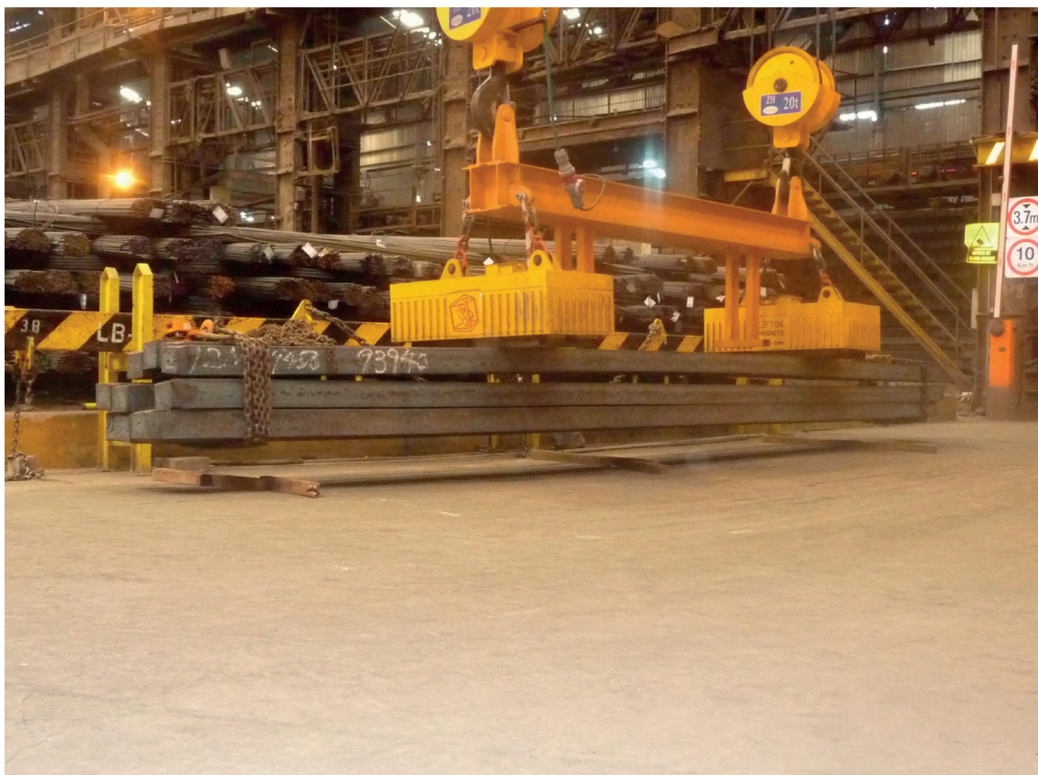
Electro Permanent magnet Hot billet lifter undergoing load test
