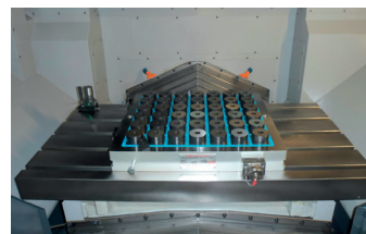
Standard 50mm Turbo Max-Mill 500 x 400 with round blocks
